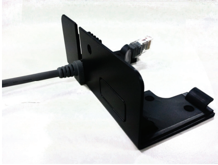
Figure 13: Position the interface cable
