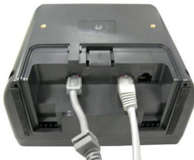
Figure 16: Insert the scanner cable and the auxiliary Cable
